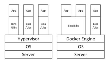
Figure 5-1. Differences between the VM and Docker container
